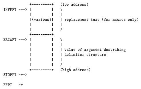
The code labelled EVTREE and subroutine GETDEL build up the new delimiter structure at the top of FSTACK. There is a block of information, the ALL block, associated with OPT-ALL brackets and this block is stacked on BSTACK at each OPT and restored at each ALL. BSTACK also contains information about nodes. The entry for a node depends on whether it has been placed yet. When a node has been placed, its stack entry is:
