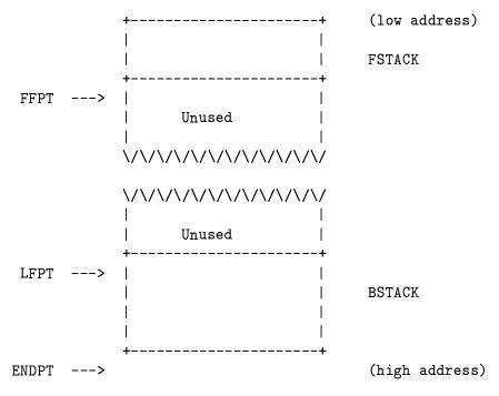
FFPT points at the first free location on FSTACK, and LFPT points at the last used location on BSTACK. If the stacks meet, the process is aborted. In general, FSTACK contains permanent information and, at the top, ephemeral text. BSTACK contains temporary information and operates as a pushdown list (the word "top" in relation to FSTACK and BSTACK means the movable end, i.e. the one described by FFPT or LFPT respectively).
