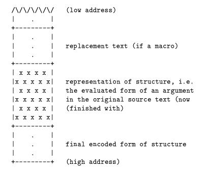
In the case of a macro, the delimiter structure is shifted up to fill in the dead space. After this has been done, the stacks have the following form in all cases. First, FSTACK:
