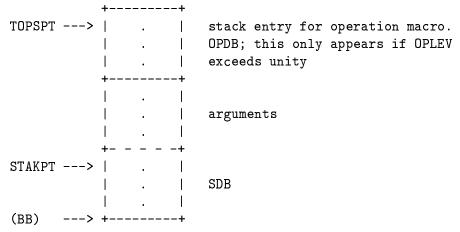
In the global case, the new definitions must be placed at (AA); in the local case, at (BB) and upwards. The latter case is quite simple. The SDB is, of course, unstacked before the new definition is moved on top of it.
