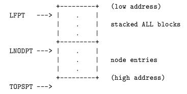
Note that when a new node entry is made, all the ALL blocks are shifted up to make room. After EVTREE has finished, the top of FSTACK is:
