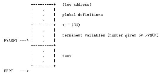
MKROOM makes space for a block of length IDLEN to be inserted at (CC). All pointers to the text that have been stacked on BSTACK are adjusted by IDLEN.
